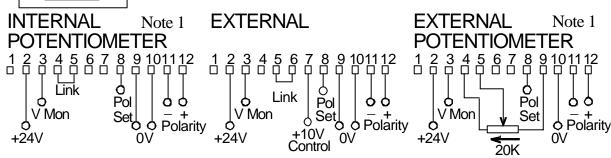
Pin 7 I monitor (if fitted). 3 Analogue voltage input 0 to +10V gives 0 to max. O/P. 2 Pin 1
